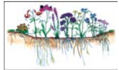
Deep rooted native plants are used in raingardens , which help stormwater infiltrate rather than run off.
